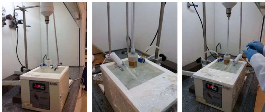
**Figuras 11a, 11b e 11c – Sistema de Sulfonação em reator**
